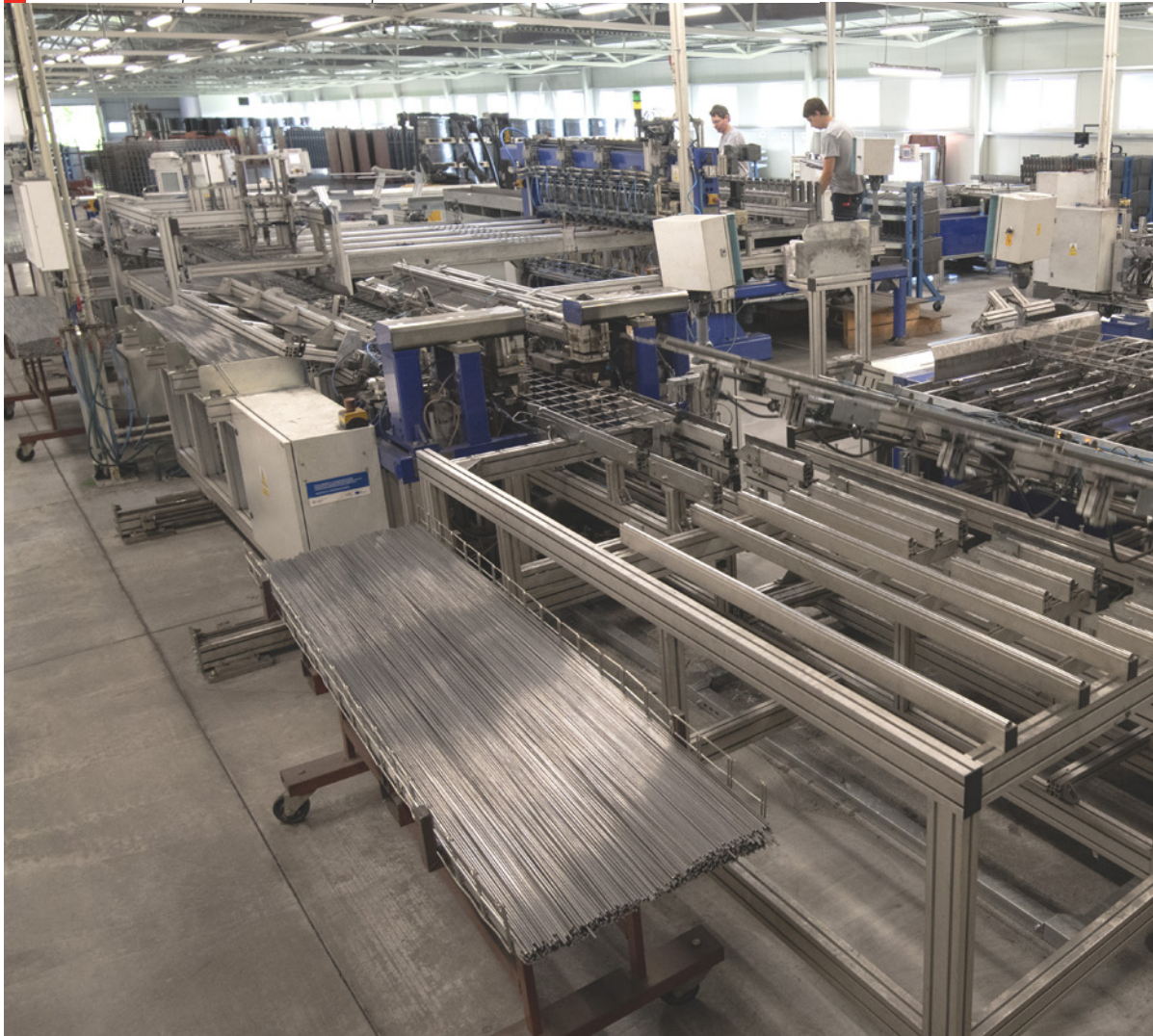
✓ Automatic line for the production of the MERKUR 2 ducts.
