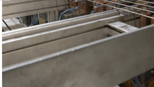
◀ ▶ Medium-frequency welding centres for welding the wire structure of MERKUR 2 ducts.
