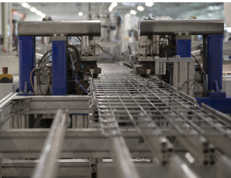
◀ ▶ Medium-frequency welding centres for welding the wire structure of MERKUR 2 ducts.
