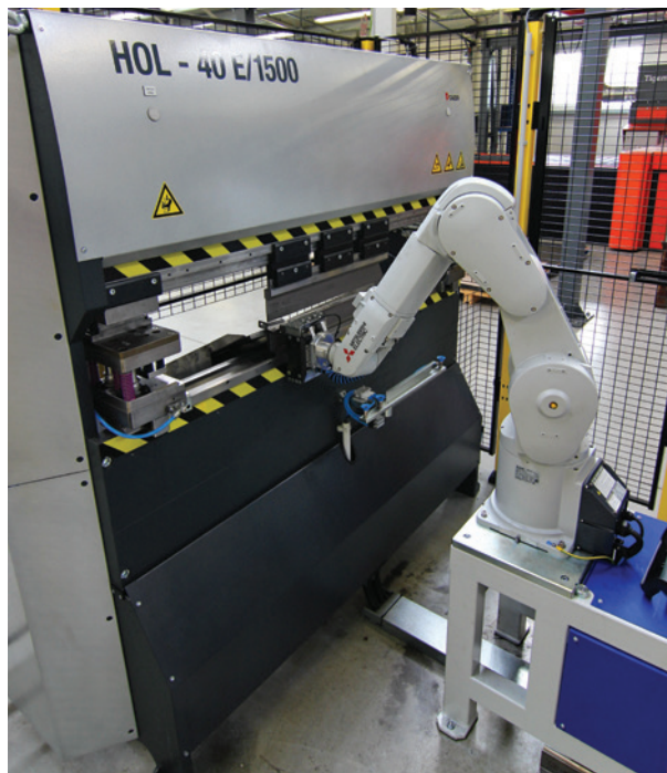
▶ One of the robotic workplaces for the production of bent sheet metal elements in the ARKYS production premises.
