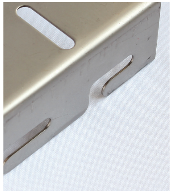
▲ A4 - stainless steel AISI 316L, stained and passivated.
